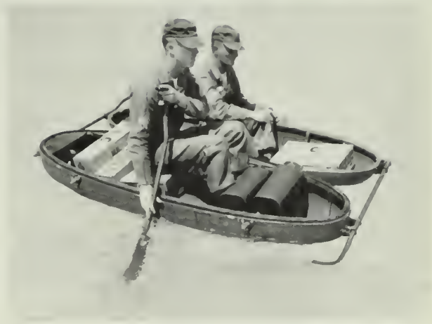
LOAD CARRYING device being tested by Army was designed for use as supply carrier for small units in normally inaccessible areas. Fiber glass cart has wide wheel for land use, can be opened into two-man boat as needed.
